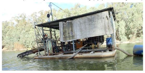
The dredges inspected varied in size from 6 metres to 42 metres long. The complexity of the dredges varied with some being manned and others unmanned, some were GPS-controlled. Thirteen of the dredges were self-propelled with the remainder being moved via steel wire cables and hydraulic winches.
