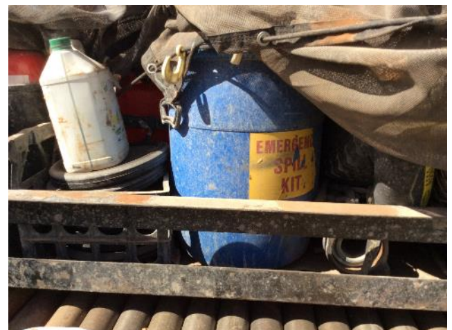
Figure 3 Spill kit in the box trailer
