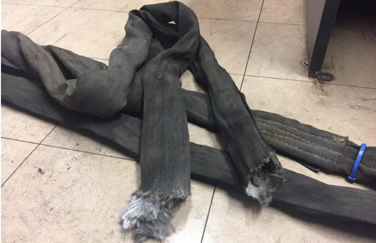
Figure 2: The failed sling
