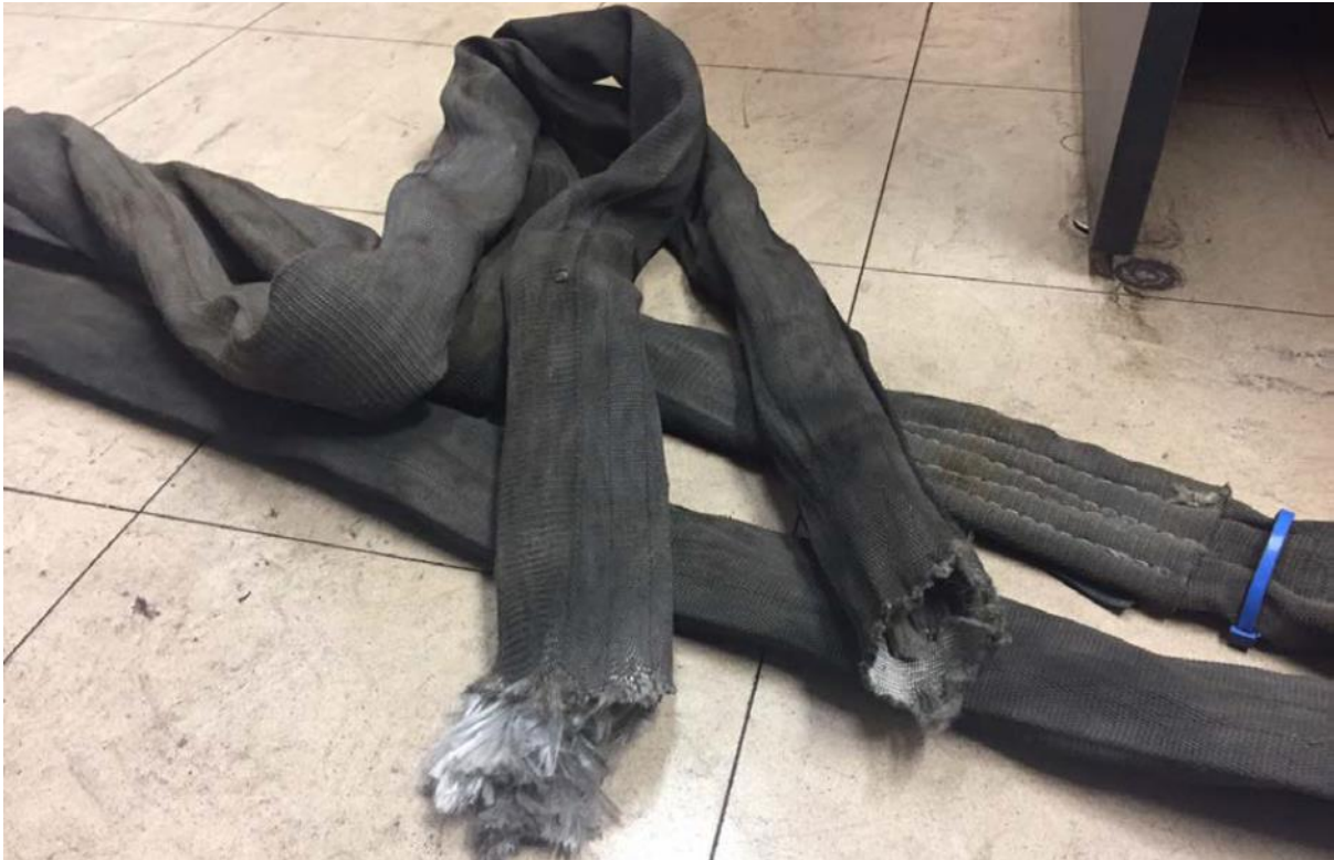
Figure 2: The failed sling
