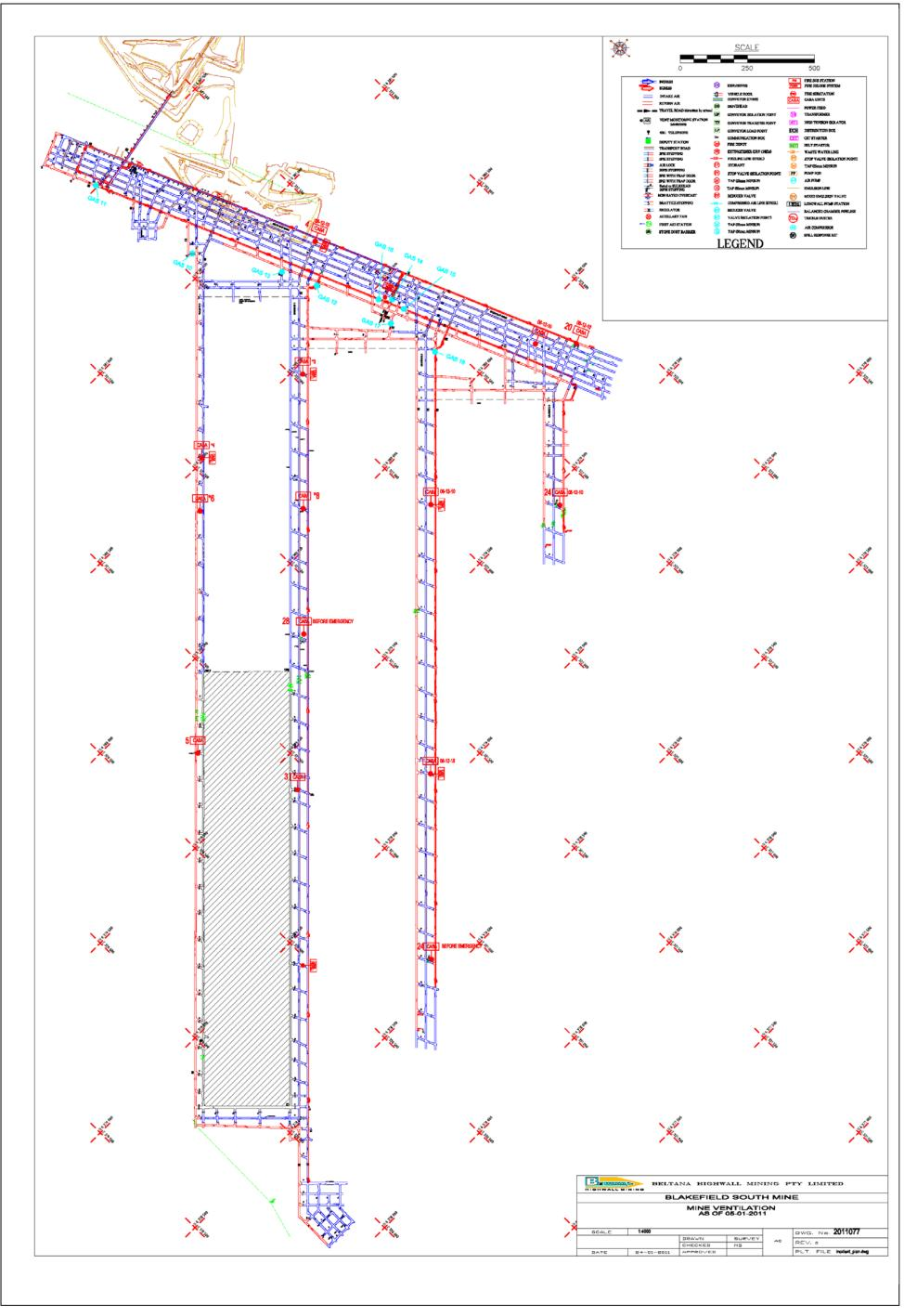
Figure 8: Plan of Blakefield South Mine showing mine ventilation and location of gas monitoring sites
