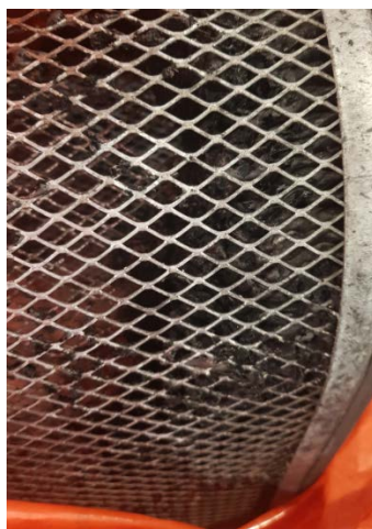
Figure 32 and 33 Tahmoor incident - melted low water shutdown floats and exhaust filter element
