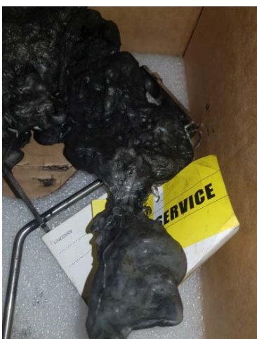
Figure 32 and 33 Tahmoor incident - melted low water shutdown floats and exhaust filter element
