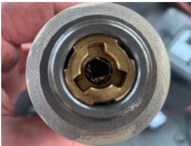
Figure 42 Mt Arthur incident, punctured fire suppression canister
