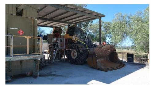
Figure 1 Volvo L220H loader with the cab in the raised tilted position
