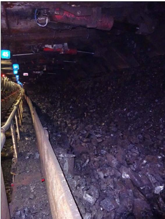
Figure 2: Ejected coal in the walkway as a result of the coal burst.<sup>ii</sup>
