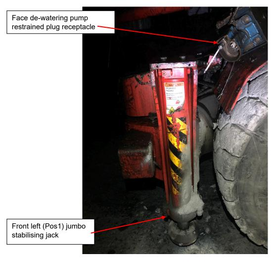
Worker receives crush injury to foot from hydraulic stabilising jack on jumbo rig
