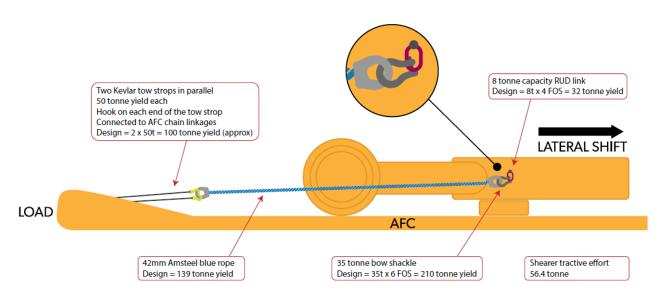
The workers began to move the AFC chain by simultaneously powering the maingate slow runner and the shearer. Shortly after starting, a loud bang was heard. The 8-tonne RUD link on the shearer failed,
