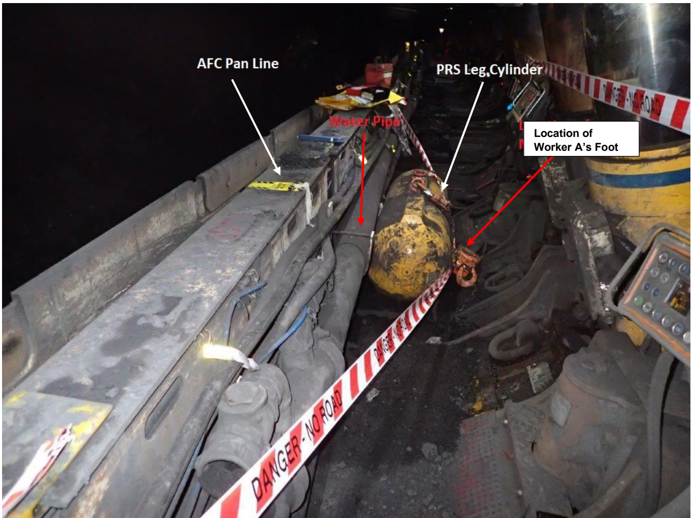
Figure 7 Photograph of PRS leg cylinder on pontoon of PRS44 following the incident, facing tailgate
