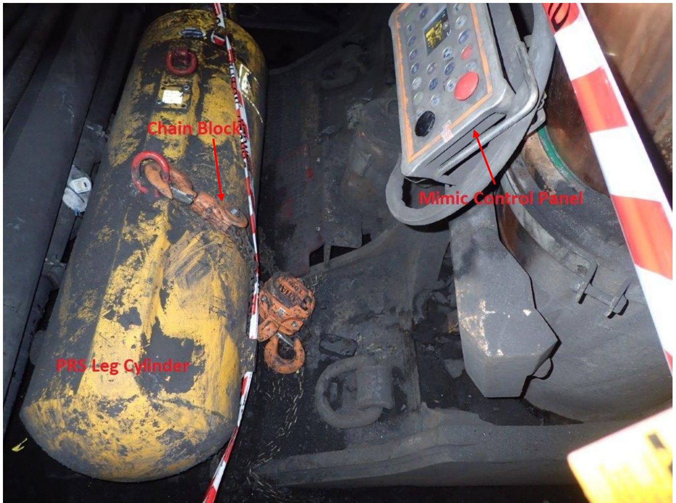
Figure 9 Photograph of PRS leg cylinder on pontoon of PRS44 following the incident
