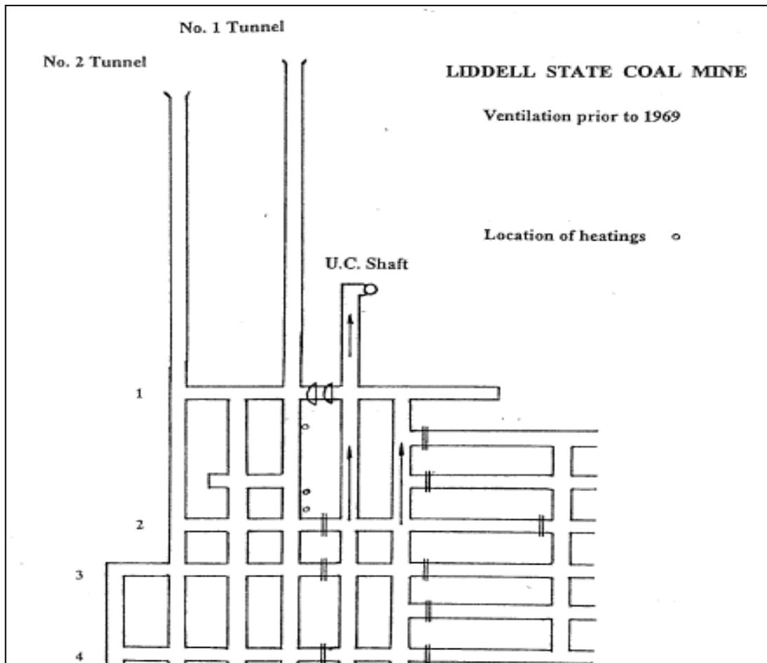
In September 1969 another heating took place in the ribside of the pillar between the intake and return. The heating was dug out and the pillar infused with water. No 2 Heading was sealed off completely between No 1 and No 4 c/t's and daily inspections and regular sampling carried out.
