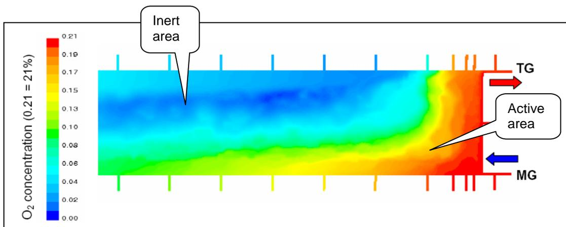
Figure 8 shows the changing goaf atmosphere as the longwall retreats away from a fixed sampling point and demonstrates that the atmosphere eventually becomes inert. Oxygen reduces, carbon monoxide initially increases due to oxidation, and then reduces as the face retreats and oxygen decreases.
