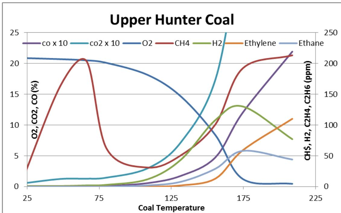
The following figures 17, 18, 19 and 20, show a comparison for several different types of coal of the evolution of gases produced by heating coal. Absolute temperature values vary but behaviour is similar.
