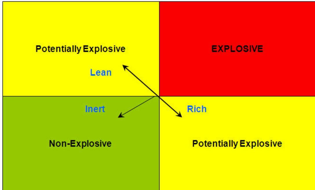
The Ellicott Diagram is a modification of the Coward Triangle that allows trend analysis. The triangle is changed into a rectangle, with the centre of the diagram being the nose point and the axes radiating from there being defined by the upper explosive limit barrier (+X axis), the lower explosive limit barrier (+Y axis), the line from the fresh air limit on the Y axis to the nose point (-X axis), and the continuation of this line to intersect the Y axis of the Coward Triangle (-Y axis).
