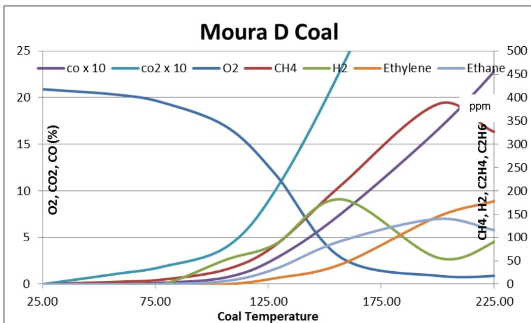
**Figure 15: Fire ladder for New Zealand coal**
