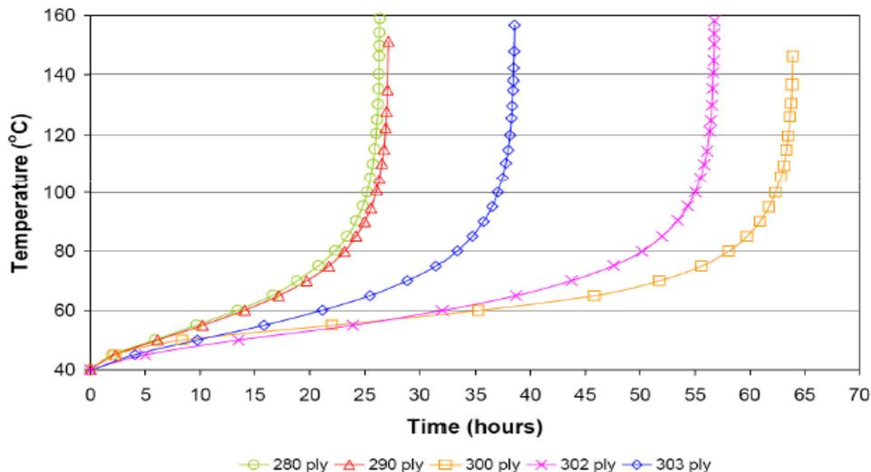
**Figure 5: Self heating relationship with ash content and coal rank for Australian coals, showing intrinsic spontaneous combustion classes (chart courtesy of Bulga Coal)**
