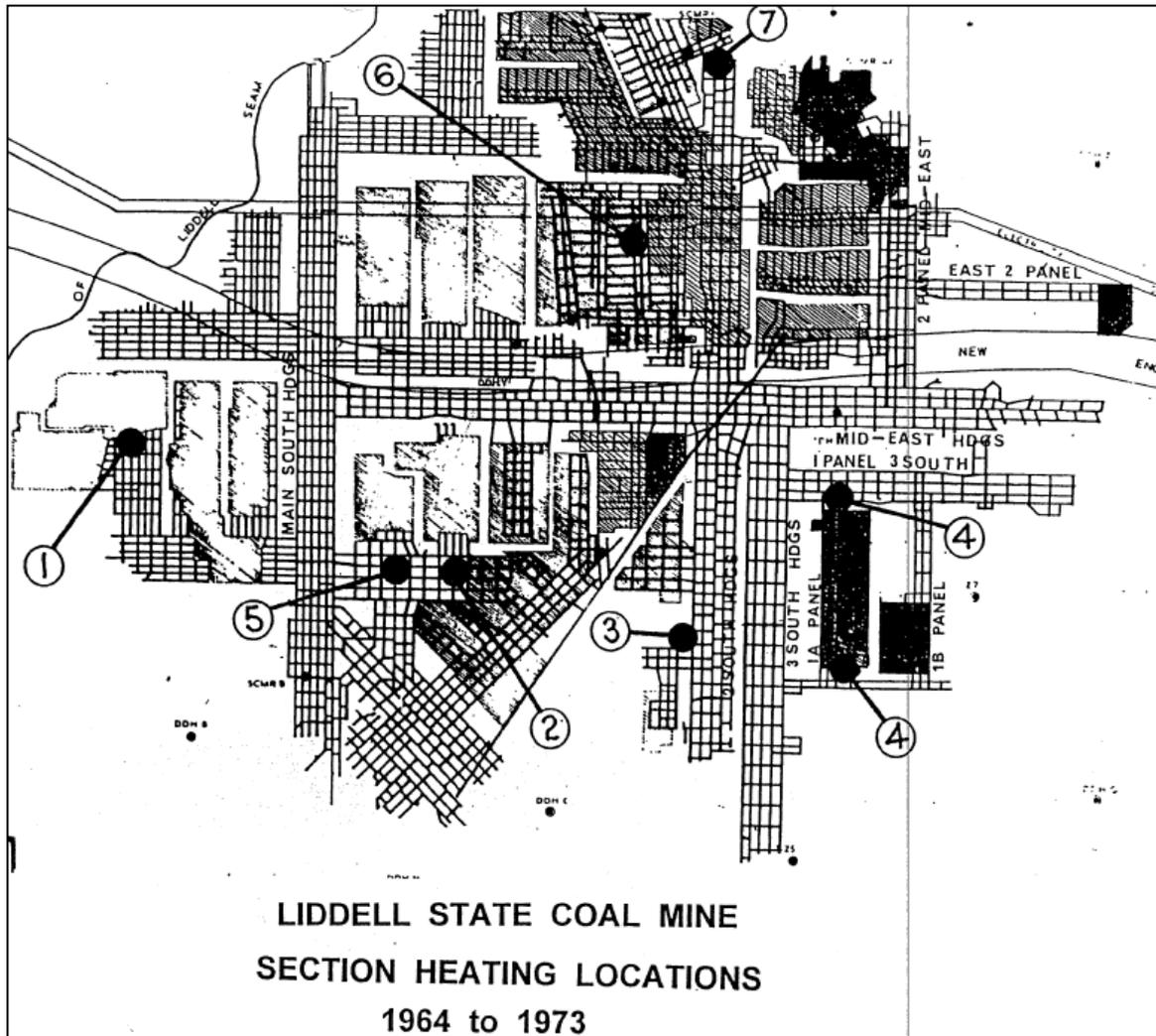
In December 1969 a new return airway was driven and the pillars between No 1 and 2 Headings were put on intake pressure (Fig 4). Inspections and monitoring were carried out on a close regular basis. For 22 months there were no indications that anything was other than normal until a fire broke out on 21 Oct 1971. The mine was evacuated and sealed.
