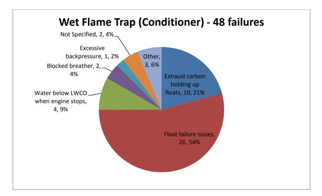
Of the 10 failures due to exhaust carbon holding up floats reported in Figure 21 above:
