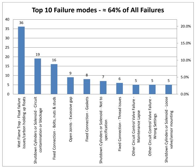
The top 10 failure modes from the 181 ExDES failures during the period January to December 2012 in the NSW underground coal mining industry are shown below:
