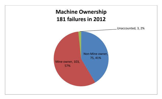
The pie chart in Figure 7 shows the contributions to the total failures from mine-owned and non-mine owned machines. The latter category predominantly comprises of machine hirers. The distribution initially suggests that mine owned machines have contributed more i.e., 57% as opposed to non-mine owned machine contribution of 41%. But, this also highlights the fact that there may be incidents that go unnoticed if they are detected once the machine is off the mine site.
