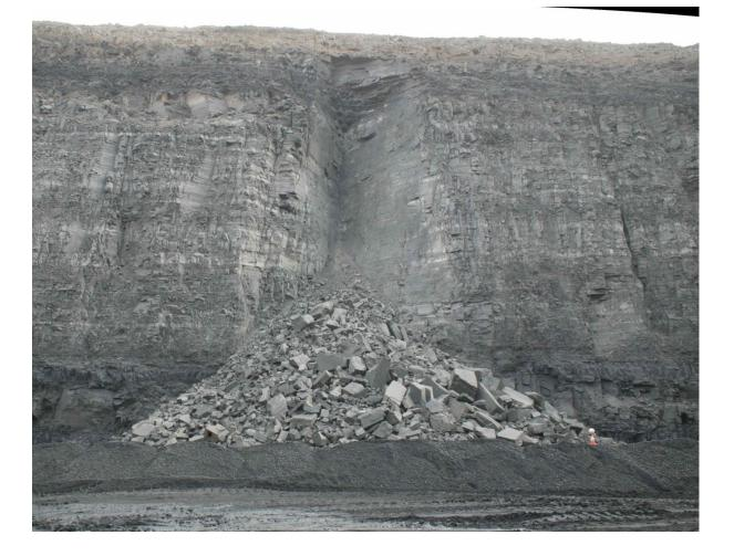
An operator has called up and informed you that there's been a major failure in the pit. This occurred when a dozer operator was pushing up a window in the area.
