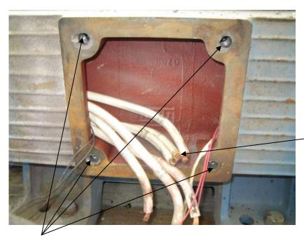
Arcing to motor leads as connection box torn off
