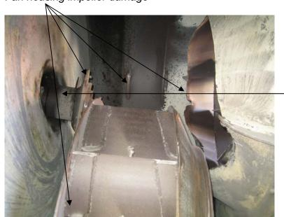
Bent motor shaft
