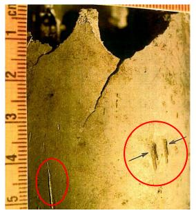
Photo 3 – Stilson marks and cracks on filter housing.
