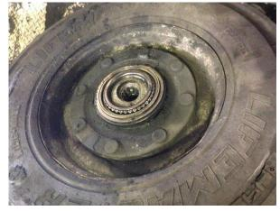
Photo 4: Failed stub axle right-hand side
