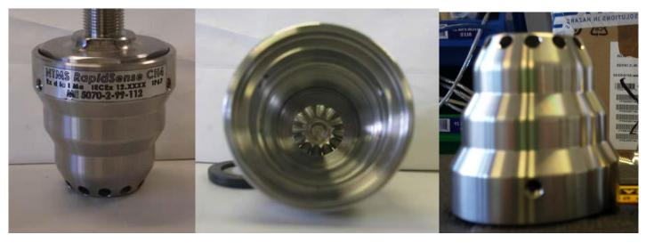
The modified housing (shown in figure 2 below) has six outside gas entry holes and a centre hole with six gas entry holes to the interior. Note also that the modified housing is taller.
