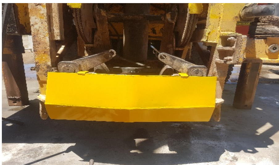
Foot clamp table with guarding fitted
