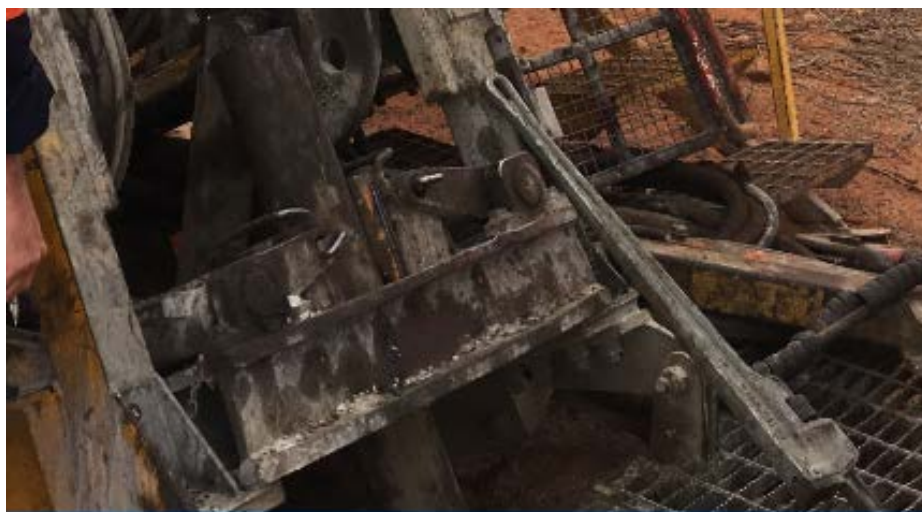
Photo 1: Foot clamp table C-section before guarding.
