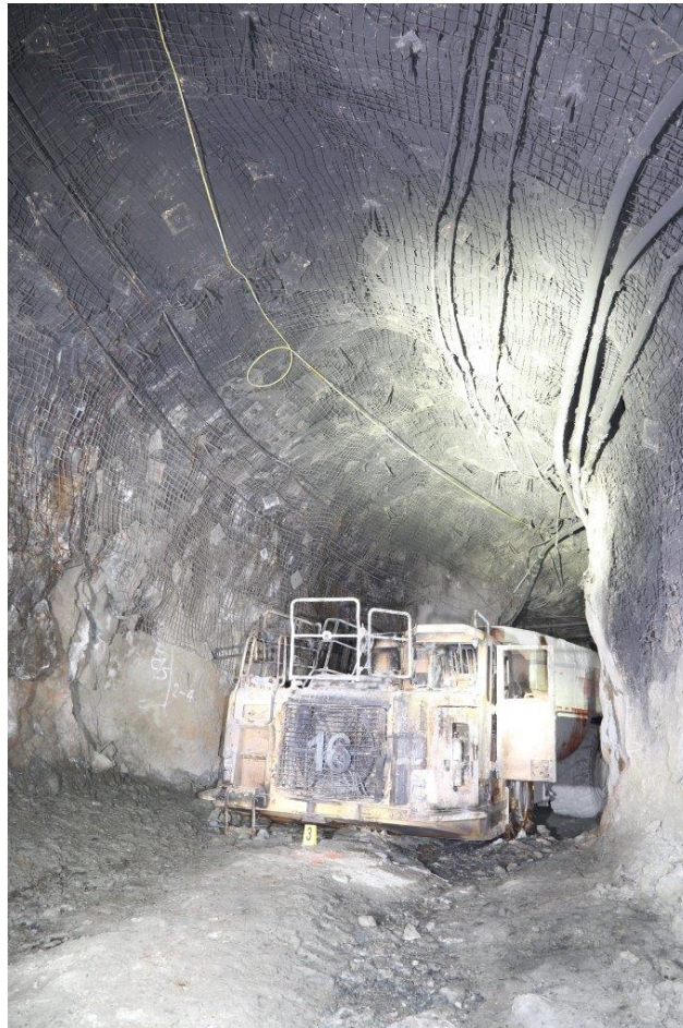
Photograph 1: Dump truck after the fire. Photo by Resources Regulator
