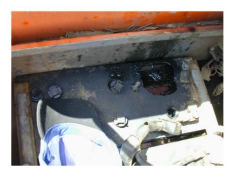
The photo shows the battery after the explosion.
