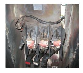
Failure 1: 630 amp 690v fuses Cat. Bussman Czech 630 NH3G-690
