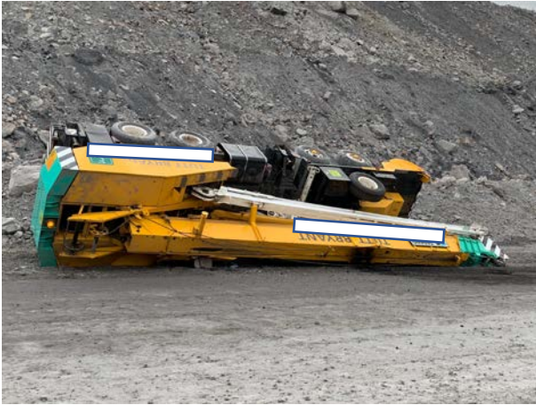
Figures 2 and 3 Incorrect use of brakes and brakes out of adjustment caused this crane to roll
