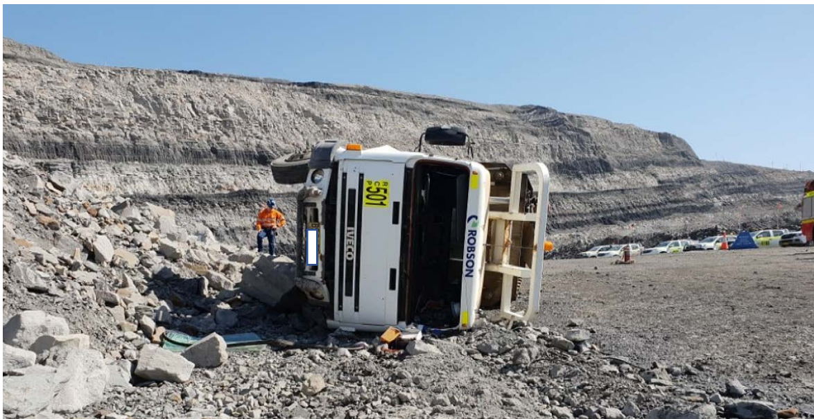
Figure 1 The truck rolled when the driver was unable to control the speed
