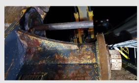
The risk of an unsecured pin falling and hitting a person is an easily identifiable risk for which controls need to be put in place prior to work commencing.
