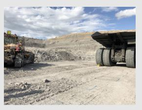
Machine operators should not rely on experience or previous movements of other operators as a substitute for positive communications. Lack of positive communication has been the root cause of many incidents and mine operators must consider higherorder controls including proximity detection. Mines should consider periodic refreshers in positive communications protocols for operators using mobile equipment.
