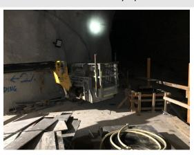
Two electricians were in a man basket attached to the extended boom of a telehandler when the basket dropped to the ground. When the boom was extended, the telehandler overbalanced causing the basket to drop to the ground and the rear of the telehandler to lift. The basket dropped approximately 3.5
