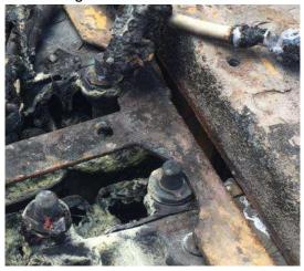
Mine operators should review their preventive maintenance inspection plans for machinery that has a battery system on board as to the standard of how the battery or batteries are retained.
