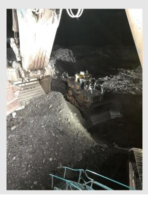
Dozer operators must maintain a safe distance when operating in close proximity to excavators (must remain outside of the excavator swing radius). Machine operators should not rely on experience or previous movements of other operators as a substitute for positive communications.
