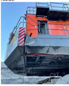
To control the risk of collision excavators should cease operation while dozers are operating within the swing radius. Mines should not rely on procedural controls for managing the risk of collisions. Collision avoidance technology should be integrated into mobile equipment.
