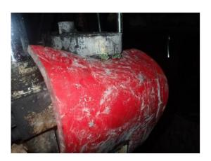
Dangerous incident IncNot0039733 Open cut coal mine While lifting a four tonne excavator slew ring from the ground, the lifting sling snapped when the slew ring was upright, allowing the ring to fall back to the ground. The lifting sling was rated for a two tonne lift and an inappropriate slinging technique was used for the lift. More appropriate lifting equipment was available at the time, including rubber sections to wrap around the load. No one was injured.
