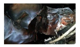
Dangerous incident SinNot-2018/00513 Two haul trucks were passing each other when one operator noticed a flame underneath the other truck. He notified the operator and immediately parked up. The fire was extinguished using a hand-held extinguisher. The centre tail shaft bearing had failed and the heat generated ignited combustible components.
