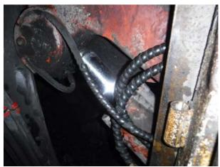
Where guarding is in place to protect workers from hydraulic release from moving hoses, the guard should be checked through the complete range of motion to ensure no gaps are present. Mine operators should manage the risk of hydraulic hoses rubbing.
