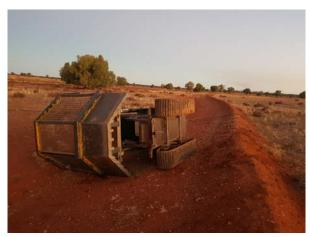
When attachments are designed, an assessment of the effects on the stability of the machine must be completed. This should be reviewed by the mine while undergoing introduction-to-site checks.
