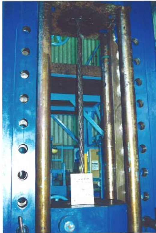
Photo No. 1Y/1 - Rope sample before testing
