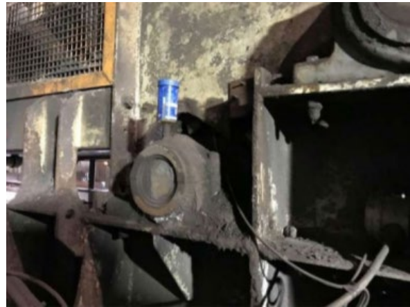
Above: The unguarded snub pulley.
