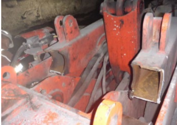
Above: Structural failure at weld point.
