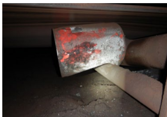
Above: The oil drum wedged under the conveyor belt.
