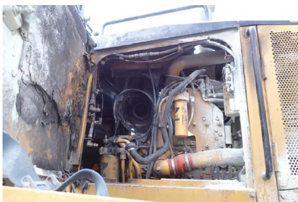
Above: The burnt engine compartment of the grader.
