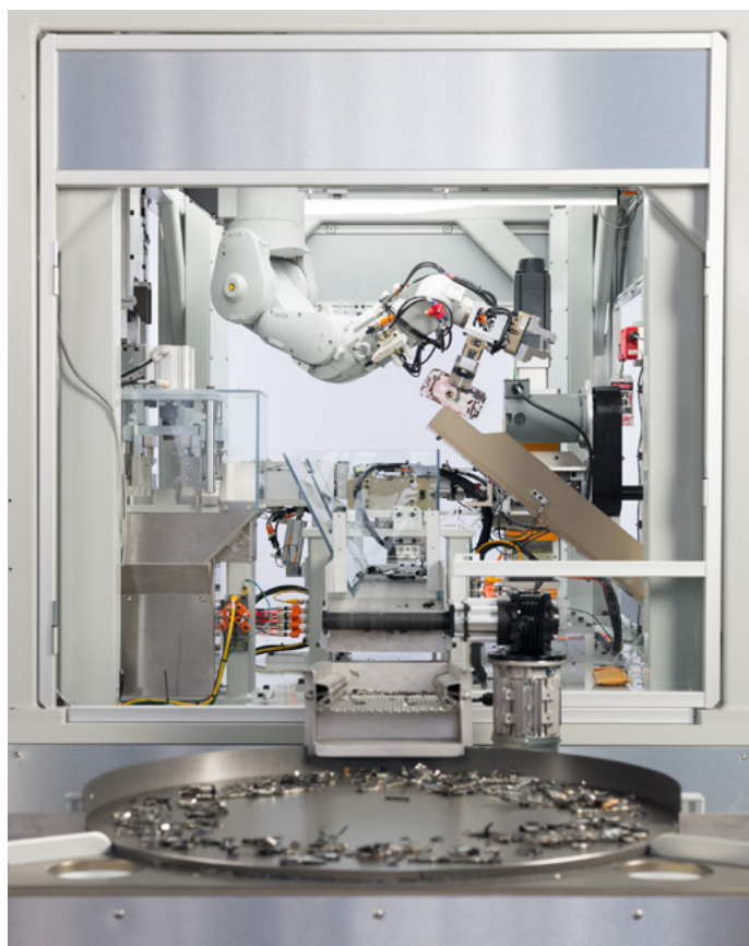
Apple's disassembly robot Daisy can dismantle up to 200 iPhones per hour. Image courtesy of Apple.
