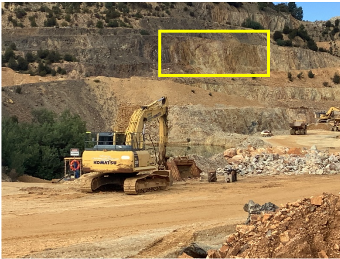
Figure 1 'Discrete' zone of material prone to generating acid mine drainage – southern face of the North-South Quarry
