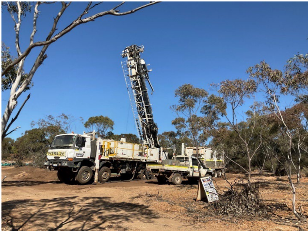
Figure 1 Diamond drill rig on hole TBD096
