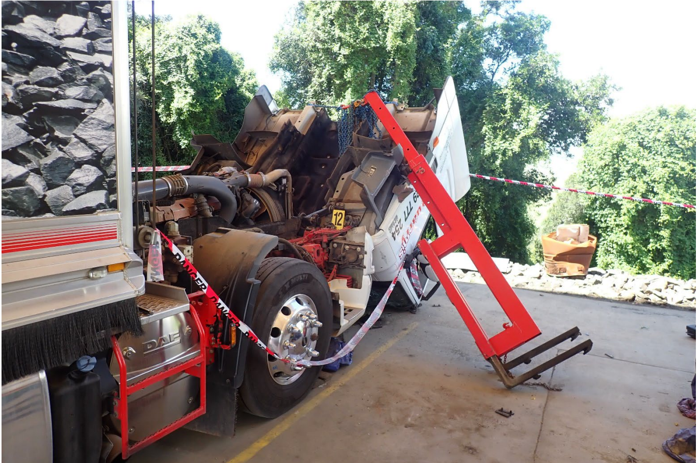
Figure 2 Position of tynes and jib following incident
