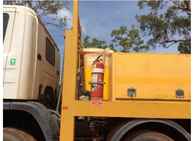
Figure 4 Yellow spill kit bin on the drill rig at 20BMDD011
