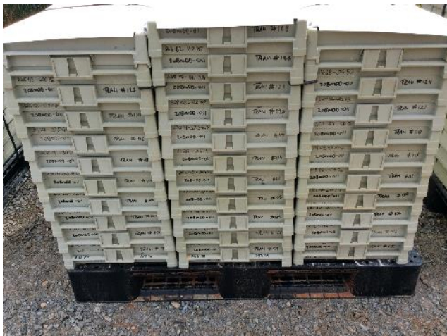
Figure 12 Core storage in modular core trays with lids
