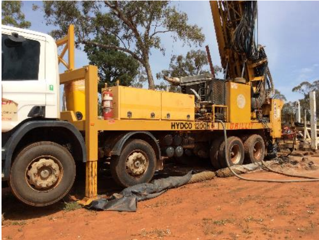
Figure 3 Rig nappy in place under the rig at 20BMDD011
