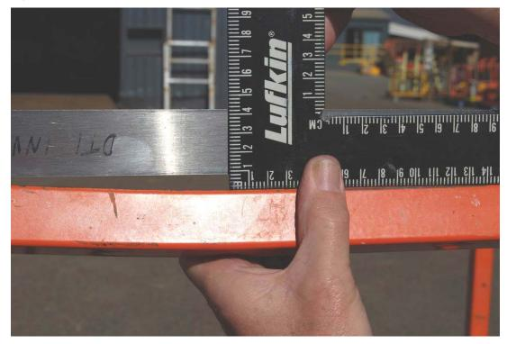
Figure 43. Measurement of the 8mm downwards deflection on the platform control console protection bar.
