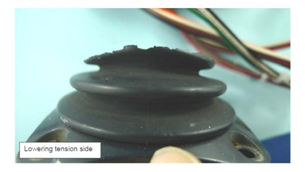
Figure 3 Views showing the multiple crack indications below the major circumferential crack on the lifting tension side, while the lowering tension side was free of any visible damage.
