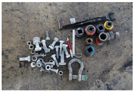
Figure 30: Photograph of items including tools rattle gun sockets, various size nuts and bolts found in the platform console storage bin and from the platform floor.
