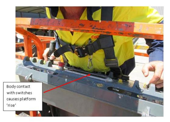
The platform lift/swing joystick control device (when the detent device is lifted on the joystick) is moved in a 'forwards' direction to achieve a 'rise' in the platform.
