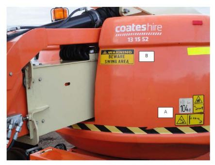
Fig 4: OEM signage provided on rear of EWP including crushing hazard (A) and Swing Area (B).
