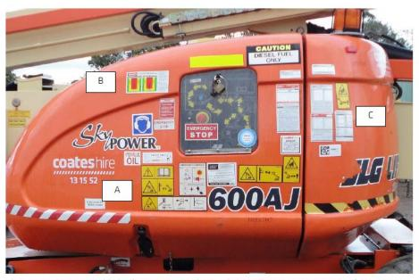
Fig 2: OEM signage provided adjacent to Ground Controls including Emergency Stop, refer operator manual, electrical hazard, tip over hazard, excessive side force hazard, crushing hazard and Emergency Control operation.
