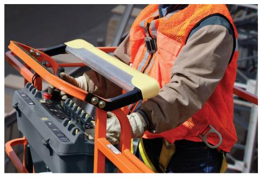
Figure 3: JLG SkyGuard® secondary protection device fitted above a JLG platform control console. ADR received for SkyGuard® by JLG on 31 May 2014.<sup>8</sup>
