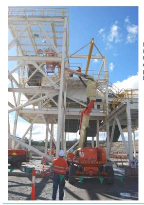
Figure 37: Platform, jib, fly boom and base boom position in relation to the turntable of the MEWP and ST202. Photo taken while lowering of the platform from the ground control box of the MEWP on 23 May 2014. Spotters were positioned on the second floor walkway and on the ground level during the lowering of the platform.
