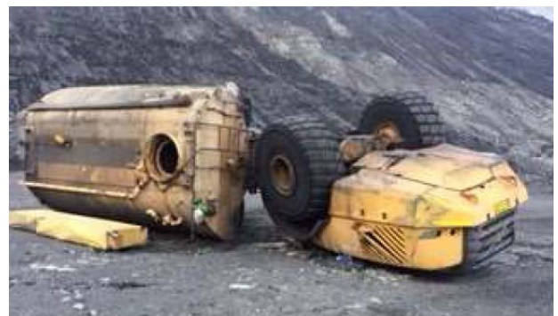
Figure 1: Articulated water cart roll-over
