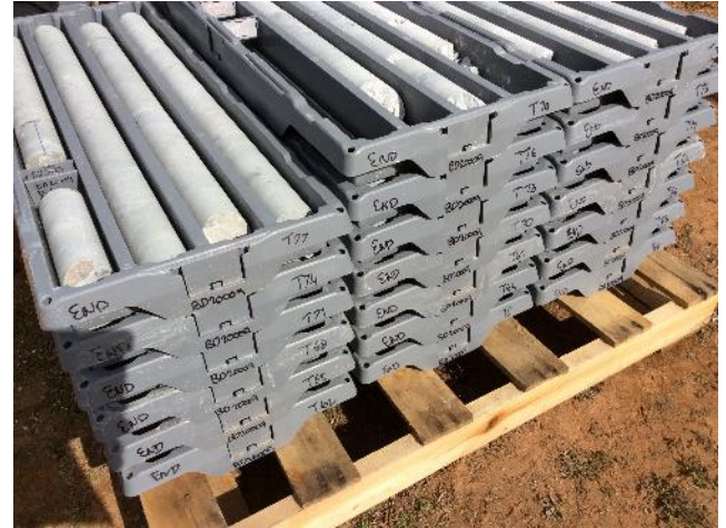
Figure 11 Example of core tray labelling
