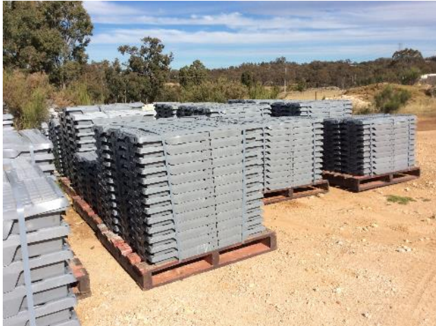
Figure 9 Core trays stacked on pallets in the core yard
