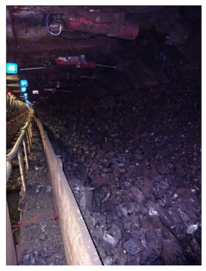
Figure 2: Ejected coal in the walkway as a result of the coal burst.<sup>ii</sup>
