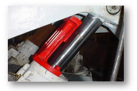
**Note:** Load-locks and other hydraulic componentry for example cylinders can fail. Hence the need for a mechanical stops as shown in the picture above.
