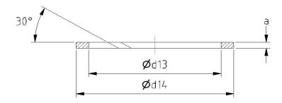
**Table 6.** O-Ring Back-up washer (all dimensions in millimetres)
