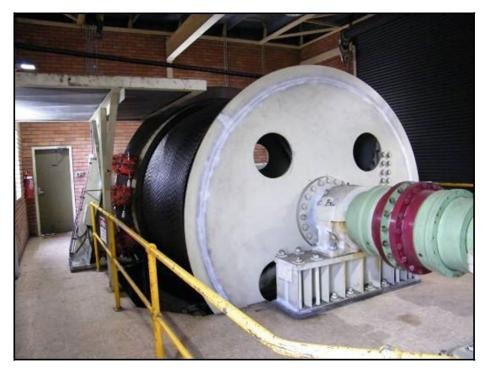
Figure 7 Coupling end shaft connection for 80 tonne drift haulage
