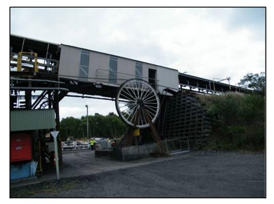
Figure 12 Fabricated and machined headsheave
