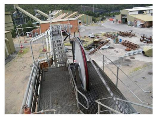
Figure 13 Headsheave installation - shaft winder
