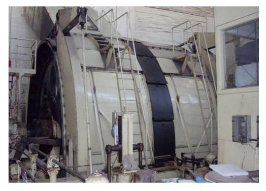
Figure 9 Alternate view of a double drum shaft winder
