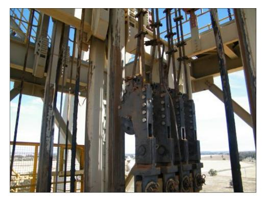
Figure 7 Examples of multi-rope suspension systems
