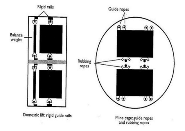
Figure 6 Guide methods used for conveyances
