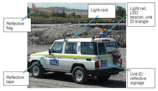
The Xstrata operators manual (used at the mine) for generic light vehicles, stated that light vehicles were essential to the smooth operation of the mine. They were used primarily for transporting personnel and operators to and from the place of work for deployment, crib times, and for changing machine operations.
