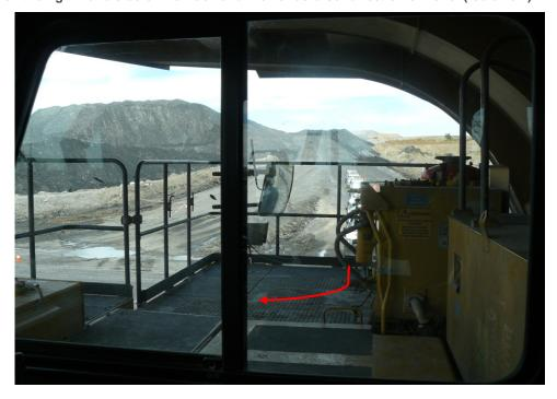
Figure 16. Photograph taken by investigators on 5 December 2013. The light vehicle is positioned in the truck's blind spot on the right-hand side of the truck simulating the right-hand turn made by Ms Forshaw.
