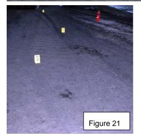
Figures 19, 20, and 21. Photographs of the tyre marks of the Landcruiser at the incident site taken by investigators at the mine on 1 December 2013.
