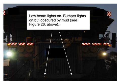
Investigators observed during the night time simulations of the incident on 5 December 2013 using the truck, that the recessed right hand side low beam light lens could not be seen from certain angles on the right-hand side of the truck.
