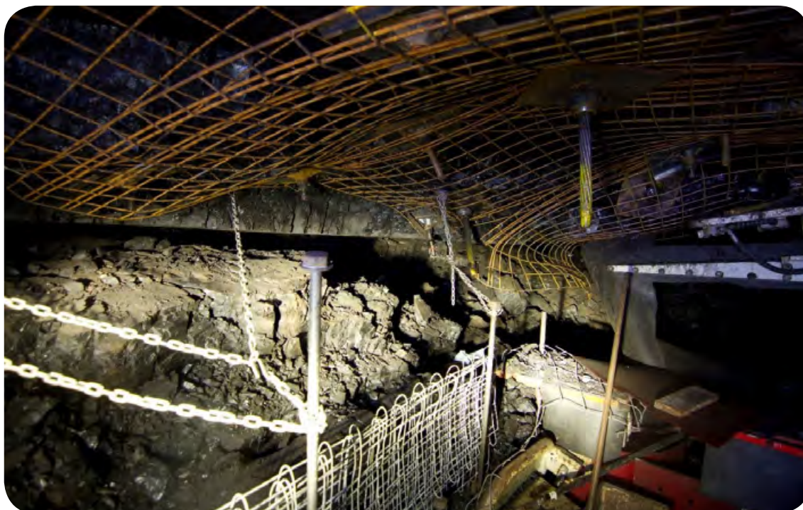
Image: Close-up of burst coal pile adjacent to the continuous miner at Astar Coal Mine, April 2014
